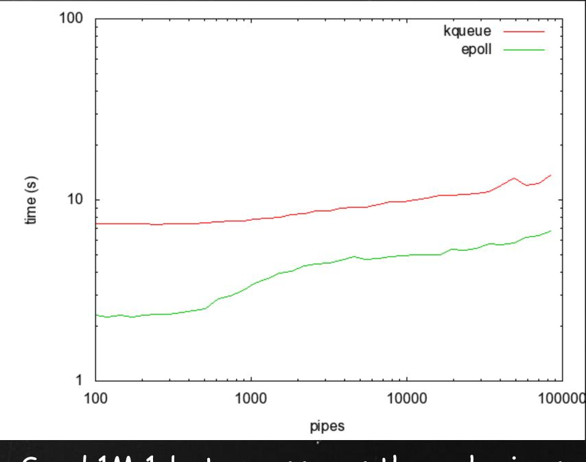
Send 1M 1-byte messages through pipes
